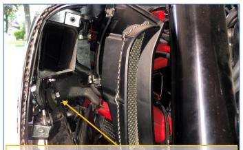
Push intake grill to the side and remove the 10mm bolt securing radiator stay to side cover.
