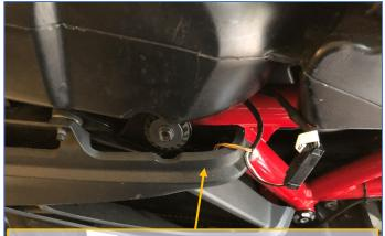
8) Connect Blinker Genie legs to mating connectors. Position connector from lamp into in retention slot.
