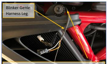
White wire on LEFT side, Green wire on RIGHT. To assist with routing, snake mechanics wire (or similar) from behind radiator support bolt up to frame area behind neck, and pull harness down.
