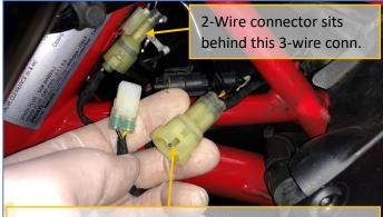
**10**) Locate the headlamp 2-wire connector attached to neck. Slide up and off of mounting tab on neck. Disconnect connector.
