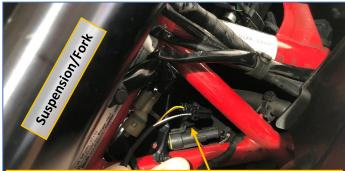
7) Rout long legs of blinker genie harness from behind steering neck area down to turn signal connectors on each side of motorcycle. Route wires inside of frame. See next image for more details.
