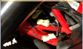
**12**) Reattach one headlamp connector to mounting tab on frame. Tuck other connector and B.G. body inside of frame
